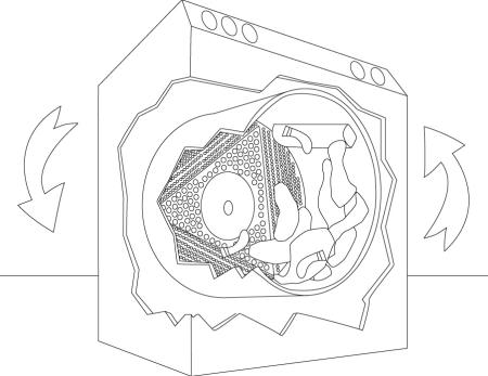
The inside of a clothes dryer spins to make the clothes tumble.
